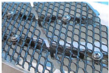
Mount the mesh using the screws. Reassemble the grill and frame by snapping them back together. If the mesh is not positioned correctly, or the mesh is too big (cut bigger than the template) the grill and frame will not fit together properly. Once properly assembled, reinstall the whole assemble back into the car.
