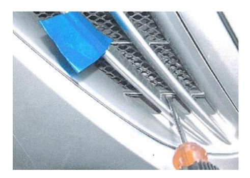
Pry the grill and frame apart at the same time you pull on the masking tape. As soon as you feel the grill pull away from the frame at that pry point, move the screw driver up to the next pry point: (photo #4).
