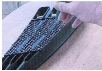
Attach the grill mesh using sheet metal screws (size #8 by ½ inch long will do. Buy at least 10 screws so you will have enough to mount the rear bumper diffuser grills, too). Washers are optional --depends on the mesh. Mesh must be properly positioned for vent and frame to snap back together-see photos #11 and 12.
