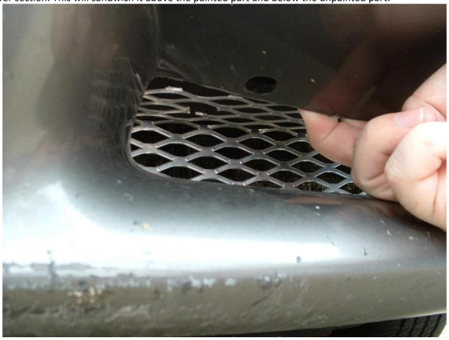
5. Push the insert forward until the holes located with the holes are lined up with the stock holes where the push screws were.
