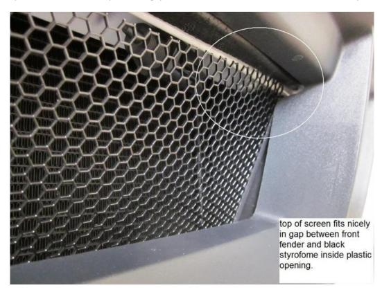
Once proper fit is found, remove mesh and apply self-adhesive mounting bases to sides and bottom of opening. No need to apply on top as the top portion of the mesh will be held in place in the gap. Two mounting bases on each side and two on the bottom are recommended.
