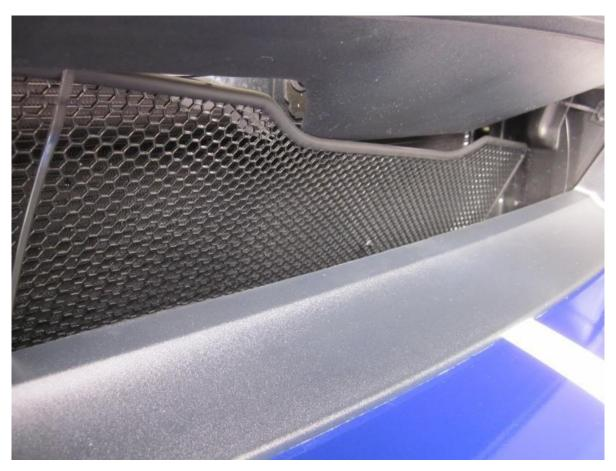
Place 3 self adhesive retention tabs on the 3 plastic tabs on inside of lower opening, 2 on top by shoulders and 1 on each side. Attach zip ties on the tabs, leaving ends open.
