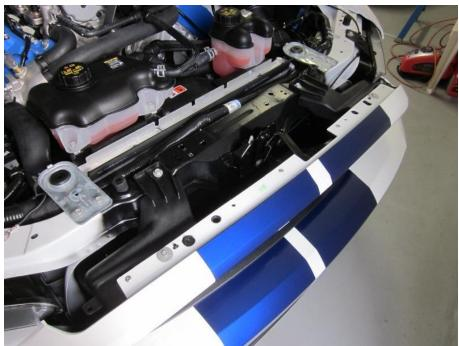
You can see into the space behind grille opening, but cannot put mesh in from above due to an attached tab from air deflector
